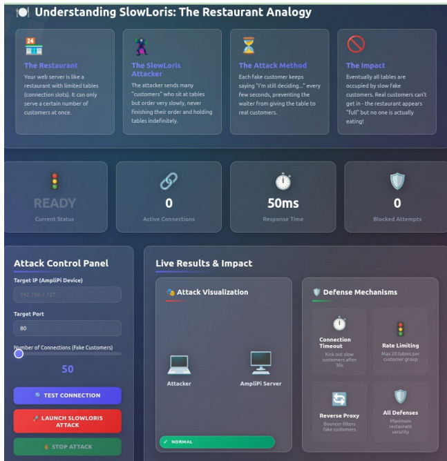
Fig. 6. SlowLoris attack tool interface showing restaurant metaphor: occupied tables represent held connections, with real-time updates as the attack progresses
